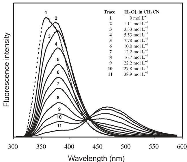
**Fig. 5.** Representative fluorescence quenching traces of **4** by added water in  $\text{CH}_3\text{CN}$  ( $\lambda_{\text{ex}}$  300 nm). Water concentrations are given in the legend. Naphtholate (**4**<sup>-</sup>) emission grows in at  $\lambda_{\text{em}}$  465 nm with increasing water content.
