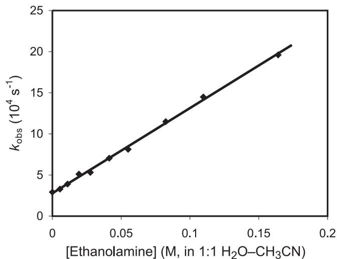
**Fig. 10.** Quenching plot showing the increase in the decay rate of **26a** at 530 nm with added ethanolamine in  $\text{H}_2\text{O}-\text{CH}_3\text{CN}$  (1:1). Line is the least-squares fit to the data and gives  $k_q = 9.0 \times 10^5 \text{ M}^{-1} \text{ s}^{-1}$ . Estimated error is  $\pm 15\%$ . Outlined point was not included in the least-squares analysis.
