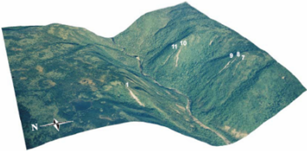
Fig. 3 3D perspective of aerial photograph 99311-67, looking east. This photograph was draped over a 5 m DEM to generate a three-dimensional perspective of the V-shaped valley form typical in Cape Breton Highlands National Park. Failure occurred on open slopes rarely associated with large-scale gullies or surface depressions. Relief in this image is approximately 400 m (Note: no vertical exaggeration). Photo Source: Service Nova Scotia and Municipal Relations, Nova Scotia Geomatics Centre, 160 Willow Street, Amherst, NS.
