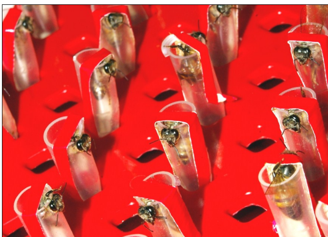
Fig. 18. Isolation cage constructed using a plastic Eppendorf tube cut in half longitudinally and sticky tape harnesses. Tube height, and outer and inner diameters = 3, 1, and 0.8 cm, respectively. Cages courtesy of CWW Pirk. Photo: V Diemann
