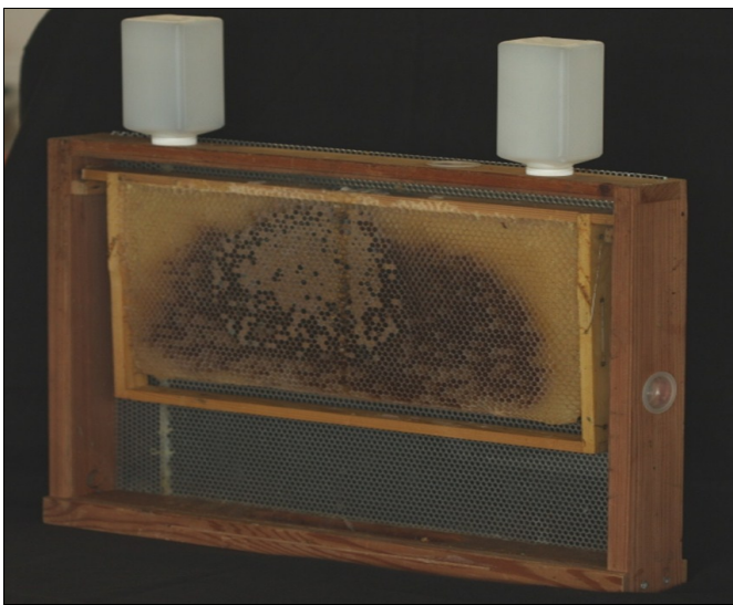
Fig. 12. A frame cage containing a Zander-sized frame and composed of a wooden casing, a metal screen, a glass removable sliding side, and two feeding devices. Cage courtesy of the Swiss Bee Research Centre.
