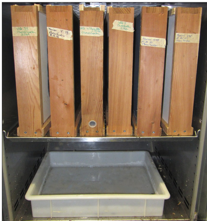
Fig. 19. Regulation of incubator relative humidity using an open water basin.
