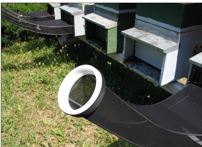
Fig. 7. Terminal end of the Bologna Trap. The ring ( i.e. , a lid with a large hole cut away) accommodates a collection container that can be attached to obtaining flying honey bees exiting the colony.
